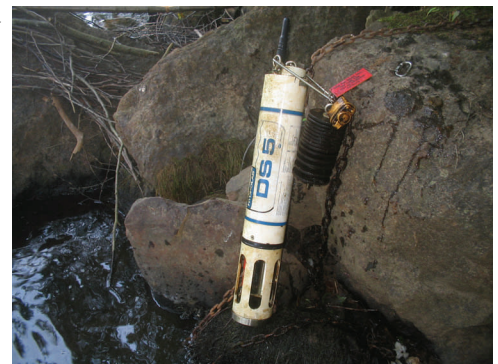
Water Quality Probe -Hydrolab DS5
